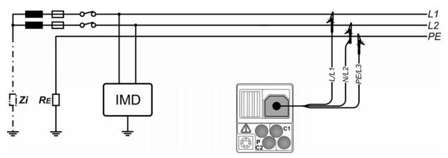
Figure 5.19: Connection for automatic measurement
