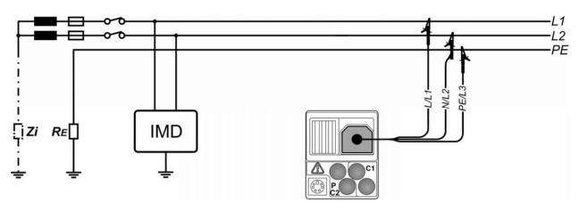
Figure 5.3: Connection of 3-wire test lead in single-phase IT system
