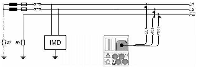
Figure 5.12: Measurement of highest first fault leakage current with 3-wire test lead
