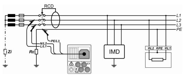
Figure 5.13: Measurement of first fault leakage current for RCD protected circuit with 3wire test lead
