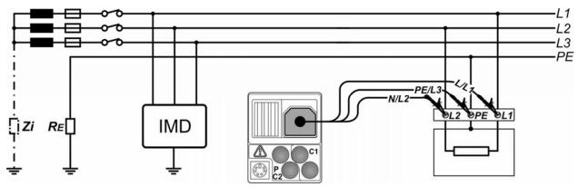
Figure 5.7: Single phase IT line impedance measurement – connection of 3-wire test lead
