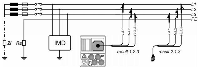
Figure 5.2: Connection of 3-wire test lead in three-phase IT system
