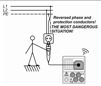
Figure C.4: Reversed L and PE conductors (application of plug commander)
