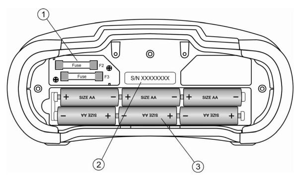
Figure 3.4: Battery and fuse compartment
