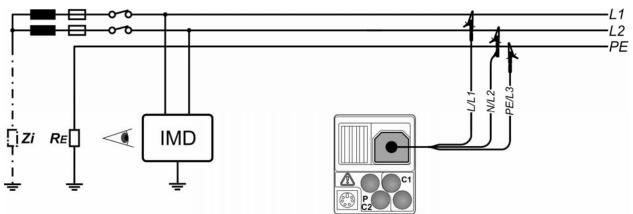
Figure 5.16: Connection with 3-wire test lead
