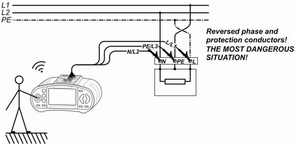
Figure 5.21: Reversed L and PE conductors (application of 3-wire test lead)
