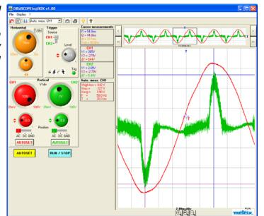
On differential channel CH1 we viewed the signal between the Phase (socket CH1+) and Earth (socket CH1-) on our distribution network, it is a sinusoidal signal with frequency 50 Hz, period 20 ms, amplitude 642 V peak to peak and rms voltage 227 Vrms
