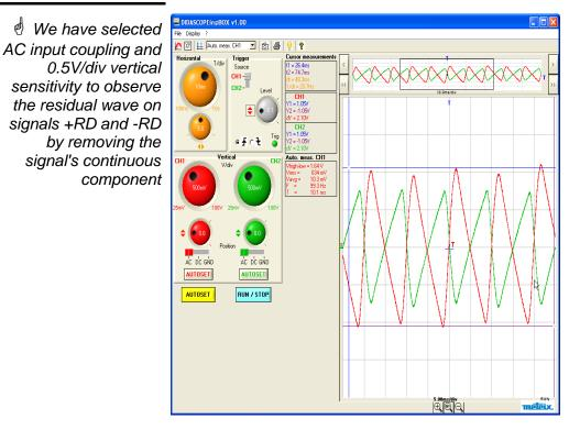
To observe the residual waves more accurately we will switch the input coupling for channels CH1 and CH2 to the AC position and increase vertical sensitivity to 0.5V/div.
