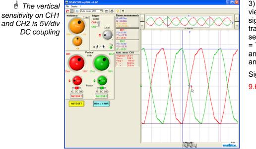
3) Simultaneous viewing of the signals on the transformer secondaries [CH1+ = T1 CH1- = Earth] and [CH2+ = T2 and CH2- = Earth]
