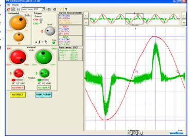
On channel CH2 the signal between the neutral and earth: is a signal with frequency 50 Hz, period 20 ms, amplitude 4.88 V peak to peak.
