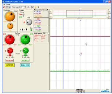
Below we show on CH1 the voltage on the transformer secondaries [CH1+ = T2 and CH1- = T1] and on CH2 the regulated voltage - 5 V [CH2+ = -5V and CH2- = Earth], to observe the residual wave after the regulator we switched the input coupling for channel CH2 to AC and selected maximum sensitivity 25 mV/div:
