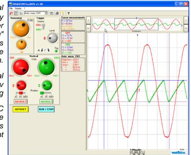
We obtain a residual wave with an peak to peak amplitude of 1.46 V approx.
