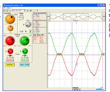
The signals at the rectifier diode terminals [CH1+ = T1 CH1- = +RD] and [CH2+ = T2 CH2- = -RD] are the following (opposite).
