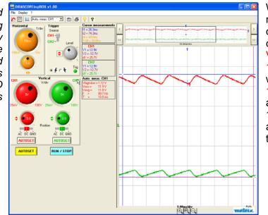
We can see that the rectified signal has a continuous component given by Vavg of approx. 11.9 V with a residual wave of amplitude 1.72 V peak to peak and a frequency of 100 Hz, because we are using "full wave" type rectification.
