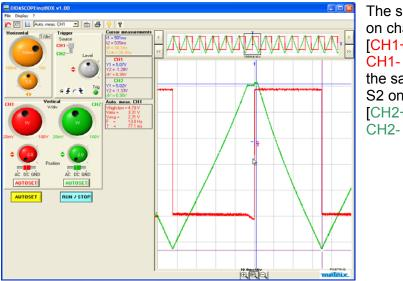
The square signal S1 on channel [CH1 [CH1+ = S1 and CH1- = Earth] and the sawtooth signal S2 on channel CH2 [CH2+ = S2 and CH2- = Earth]
