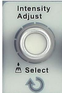
**3. Adjust Waveform Intensity/Grid Brightness/**
