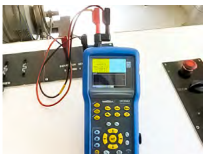
Here, channel 1 of the HandScope® is connected to the inductor via the BNC/Banana adapter.
