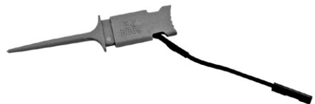
Fig. 2: Measuring cable connected with Mikrohook
