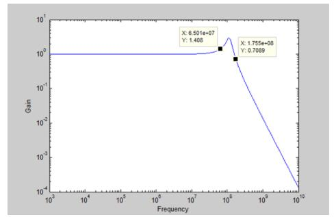
The added inductance has moved the -3dB bandwidth of the probe from >500 MHz to 175 MHz. Additionally the resonant frequency has been pushed well inside the bandwidth of the probe to 115 MHz. At 65 MHz we can still see an error of 40%, in fact, to keep the error under 10% we need to limit the frequency to 35 MHz!
