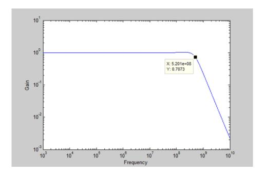
Something close to this performance can be achieved with the Teledyne LeCroy ground blade or ground spring accessories which may have an inductance of 10-20 nH. It is also important to consider the whole ground loop and connect to a nearby low inductance ground point on the device under test. Using copper foil can help to provide a nearby ground connection so that the length and inductance of the ground connection can remain small.
