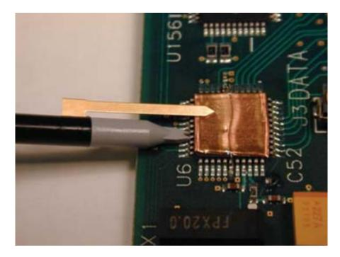
More often than not, the connection of choice is the long alligator lead. Let's investigate what effect using this ground lead has on the bandwidth and frequency response of the probe. Using this ground lead, the ground loop will have a length of at least 10 inches. Using 20 nH per inch as a rule of thumb we can calculate the inductance
