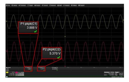
This is a 40% error in peak to peak voltage which is what is predicted by the MATLAB plot.
