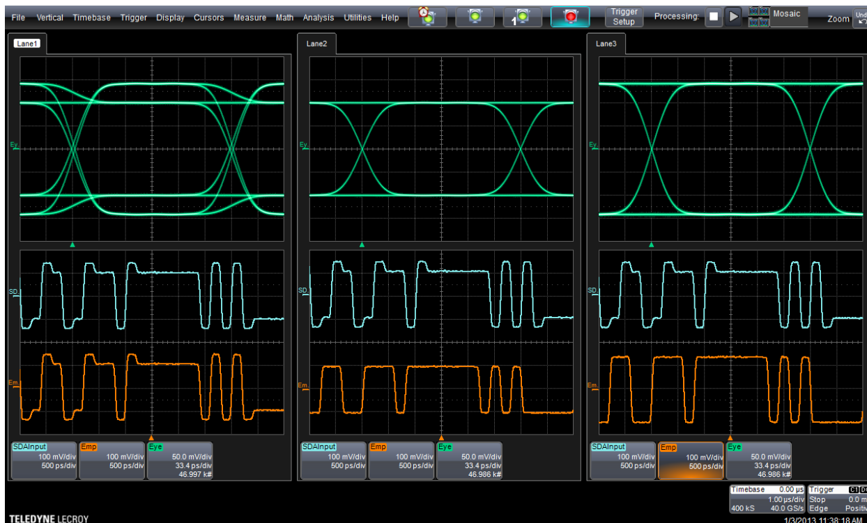
Auto-remove of pre-emphasis (center) and de-emphasis (right) along with no emphasis (left).
