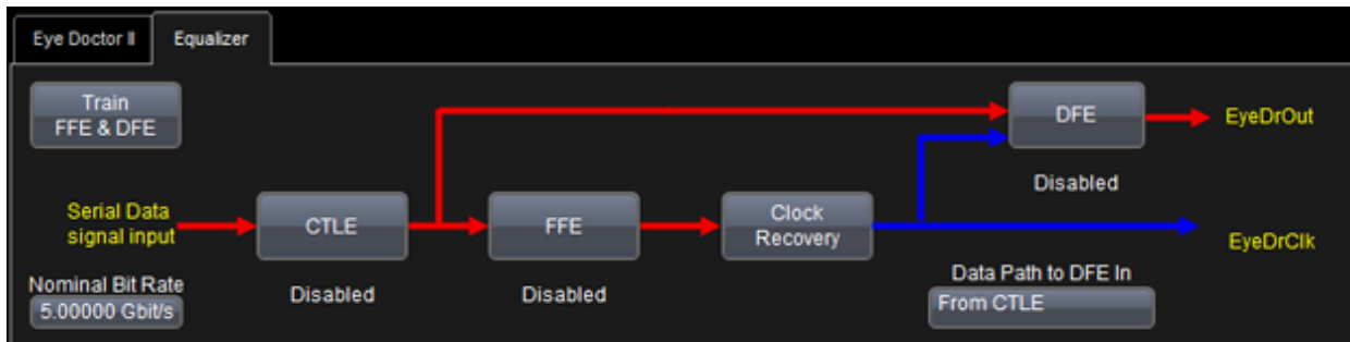
CTLE equalizer applied to data only, CTLE and FFE applied to clock recovery.
