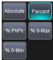
For example, if you want to set an absolute crossing level, touch inside the **Use Level Type** field and choose **Absolute** from the pop-up menu. Then, touch inside the **Abs Level** data entry field and enter the voltage level at which the signal timing is measured.
