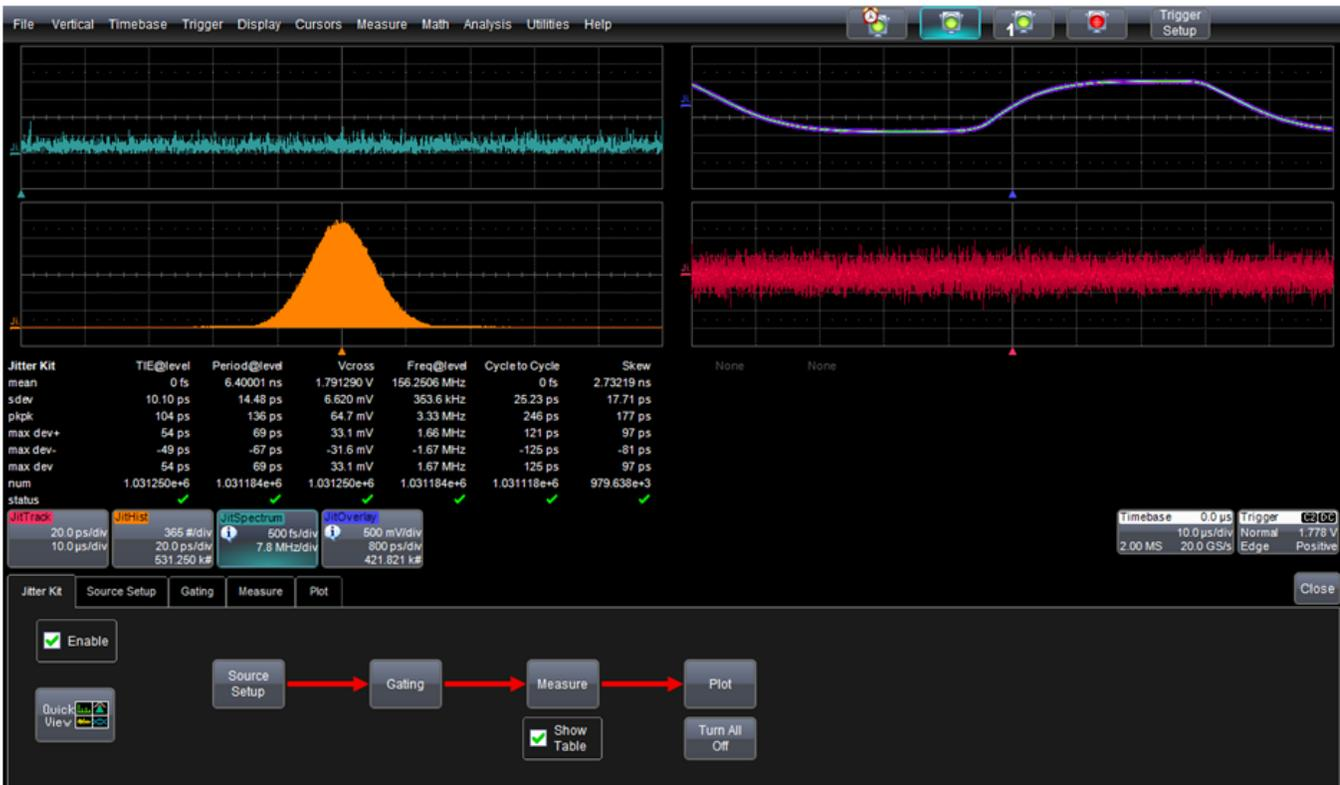
*Jitter Kit analysis of a 156.25 MHz differential clock signal including jitter measurements and views of jitter in the time, frequency, and statistical domains plus the jitter overlay*
