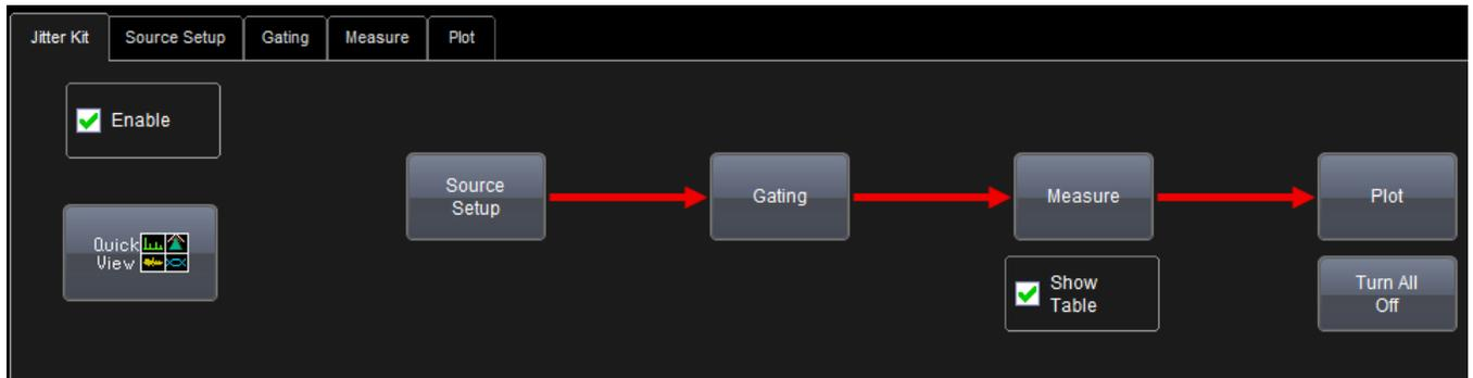
*Jitter Kit main dialog showing the basic flow of jitter analysis*
