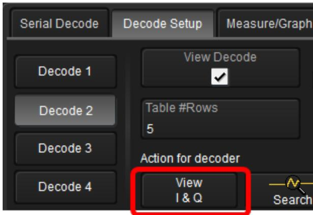
This feature enables you to generate a constellation (XY) diagram from the converted I and Q signals. The diagram appears next to the decoded waveform.
