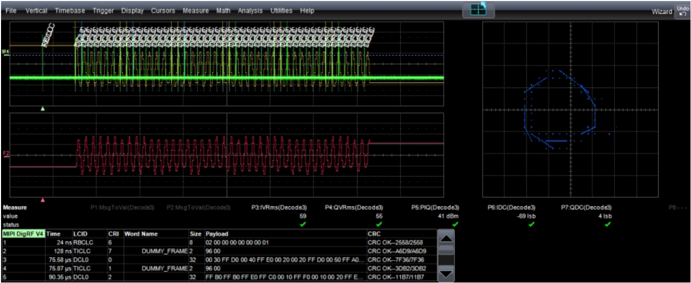
DigRF v4 I and Q display available with the -DMP option.
