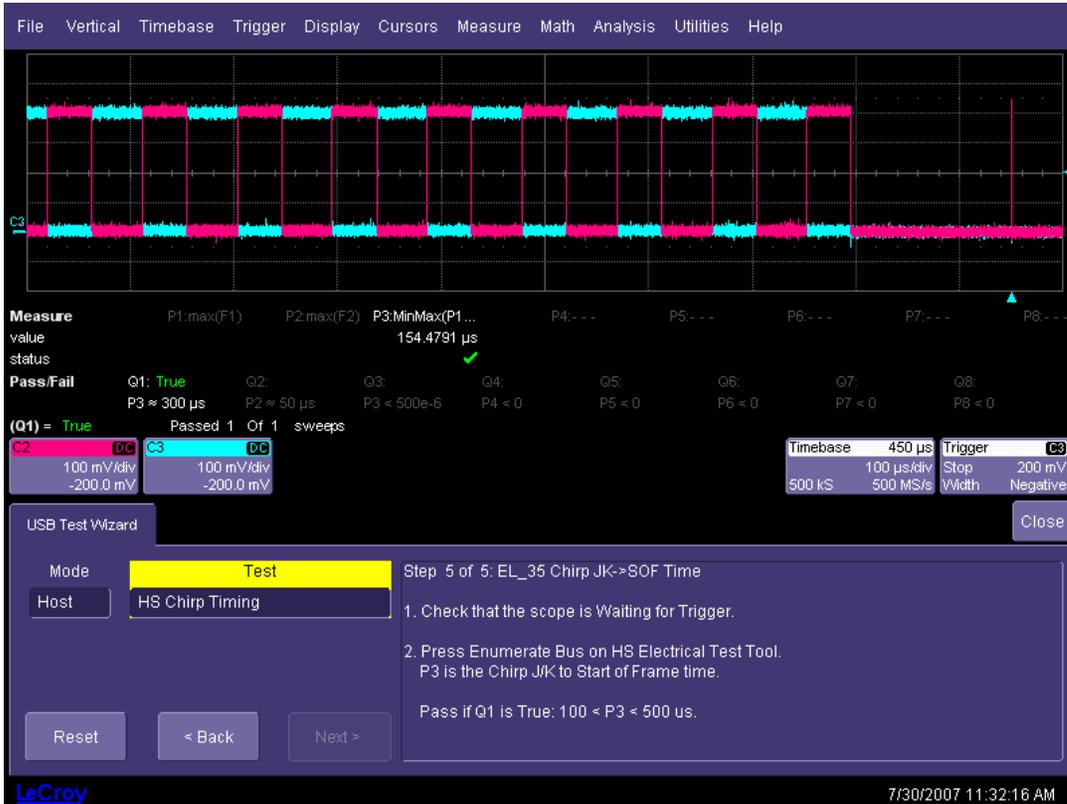
**Figure 29. Chimp to Start of Frame Time**
