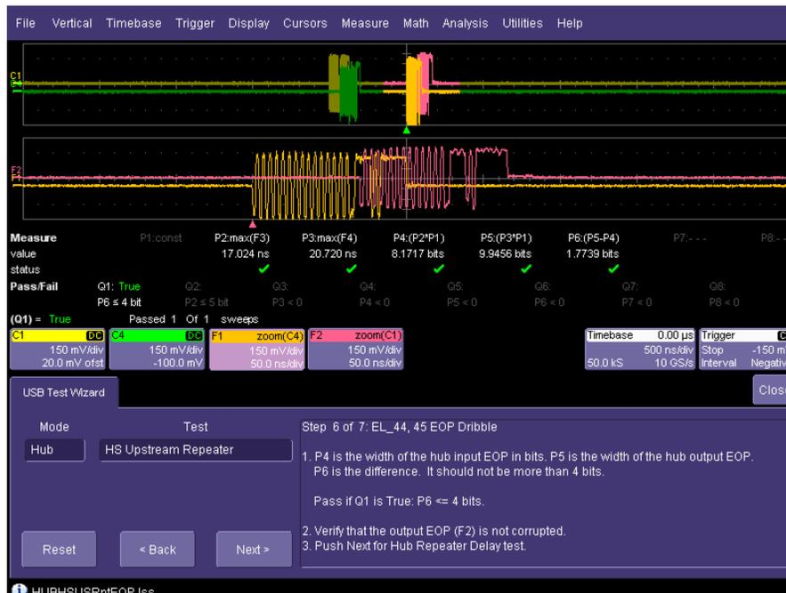
**Figure 39. Hub upstream repeater end of packet dribble**
