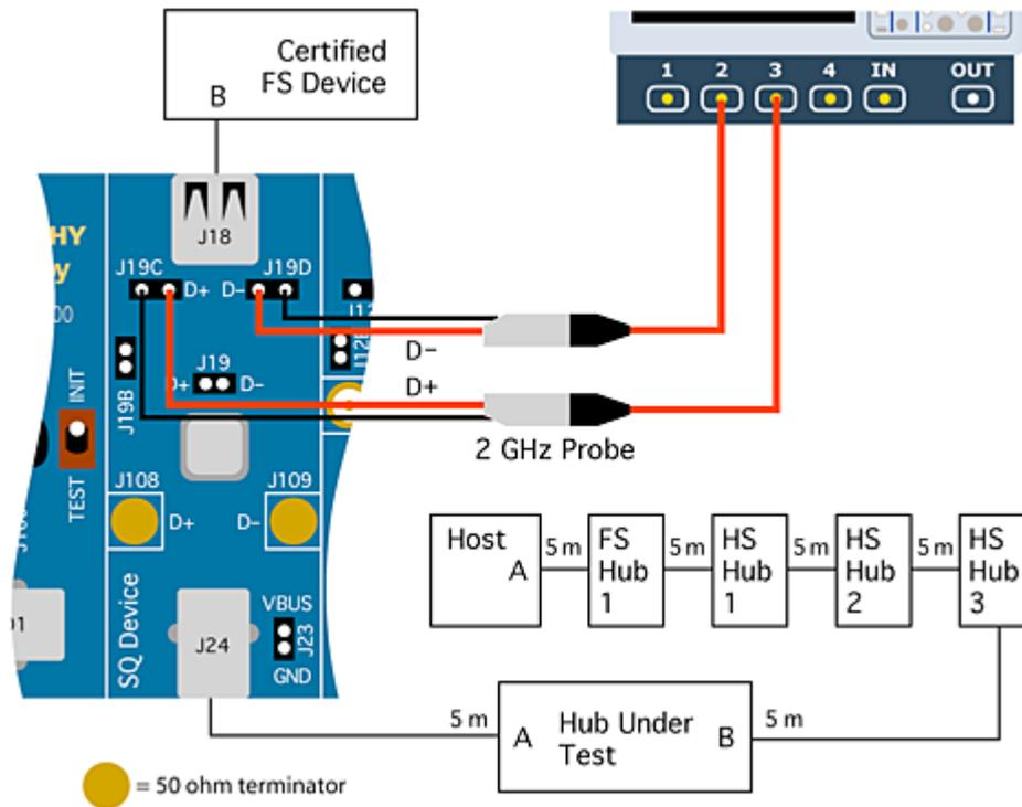
**Figure 61. Hub Full-Speed Downstream Signal Quality Setup**
