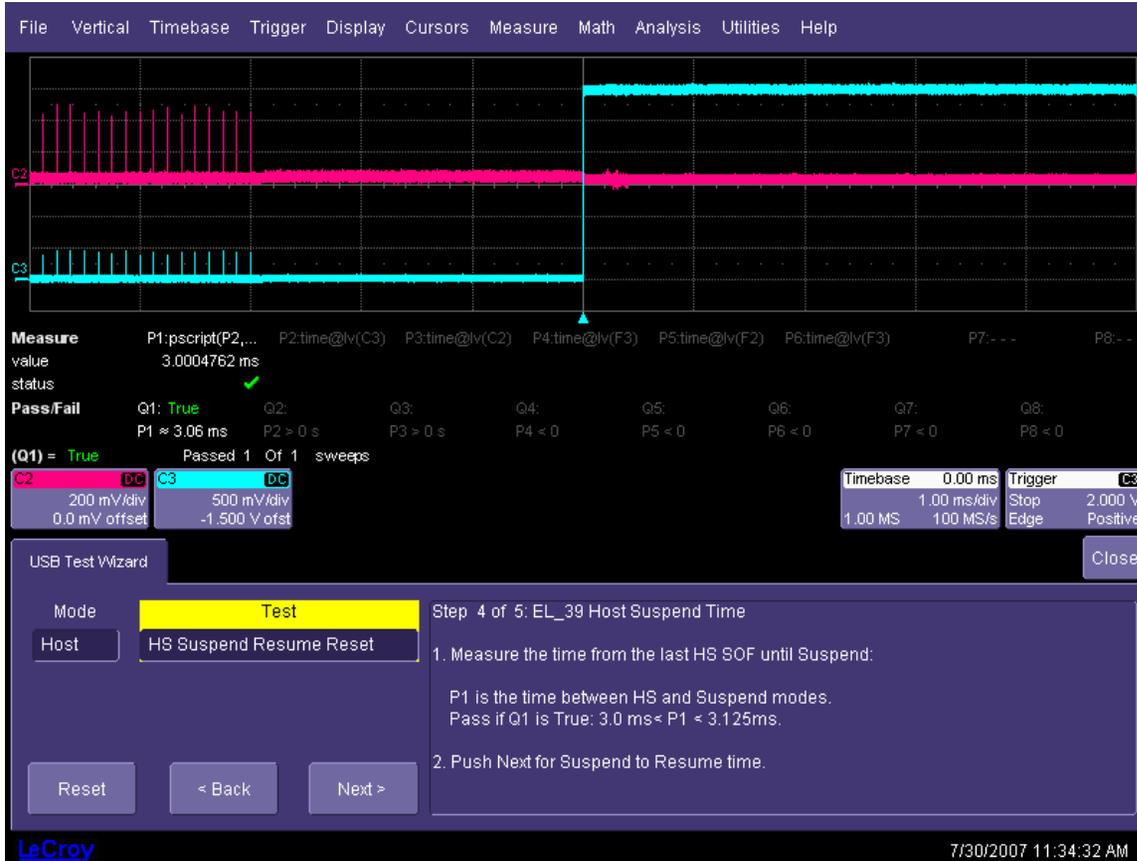
**Figure 31. Time from Last Start of Frame to Host Suspend**
