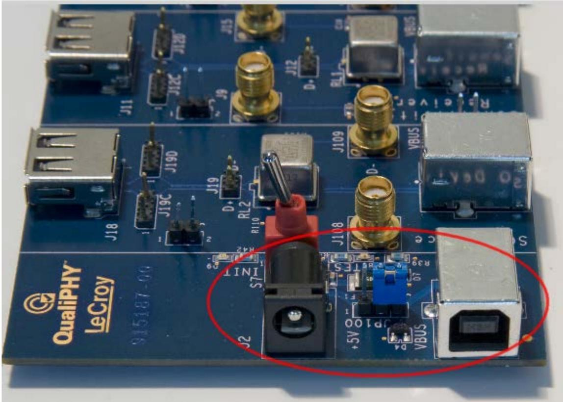
Figure 3. TF-USB-B Showing Power Supply Selection Jumper
