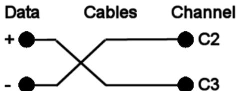
5. Write down the mean skew value after it stabilizes. This mean skew value is the addition of (-Data skew) + cable skew + channel skew.
