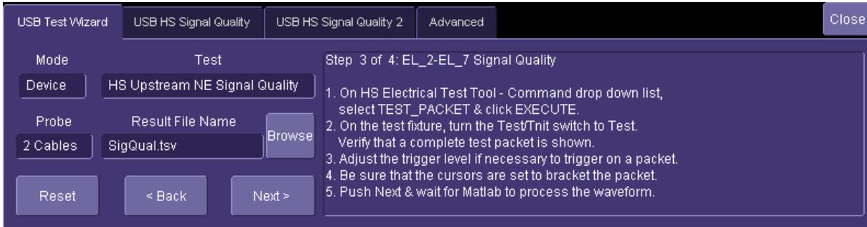
**Figure 21. Step 3 of 4: EL\_2-EL\_7 Signal Quality**
