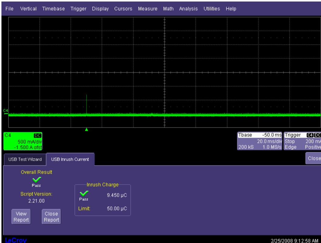
**Figure 59. Inrush Current Pulse**
