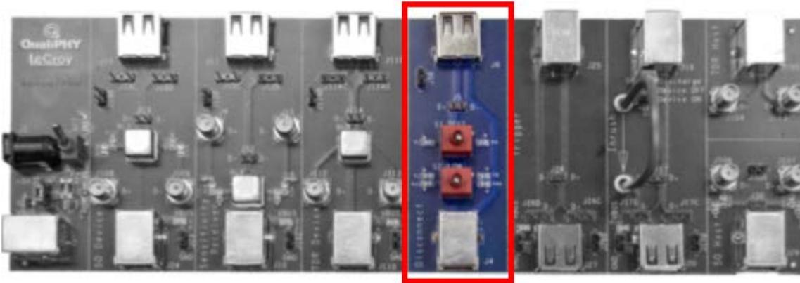
**Figure 33. Host Disconnect Section of Test Fixture**
