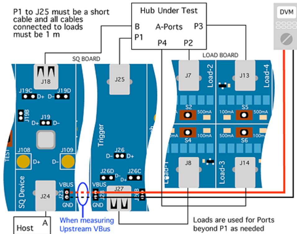
**Figure 51. Bus-Powered Hub Drop test equipment setup**
