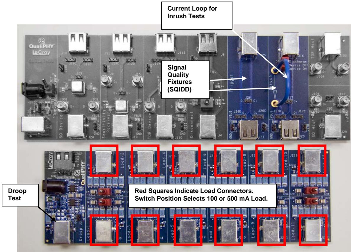
Figure 50. FS/LS Signal Quality Test Fixture Sections
