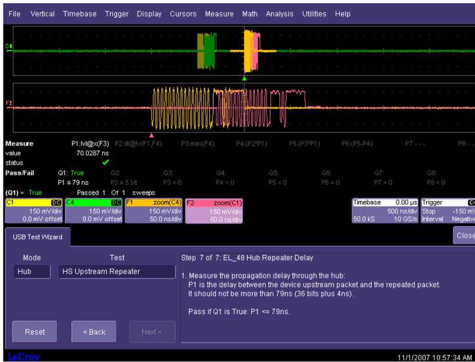
**Figure 40. Hub upstream repeater delay**
