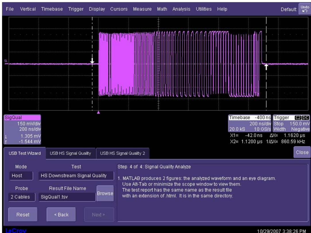
Figure 24. Host High-Speed Downstream Signal Quality Analysis
