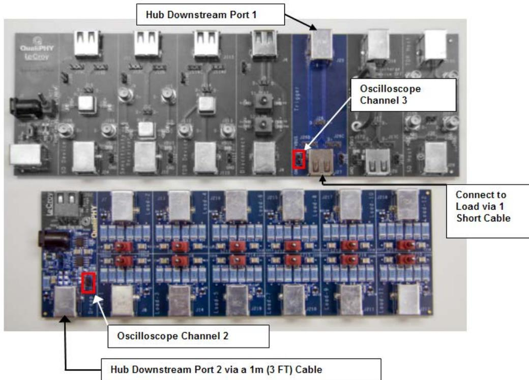
**Figure 53. Device and oscilloscope connections for droop test**
