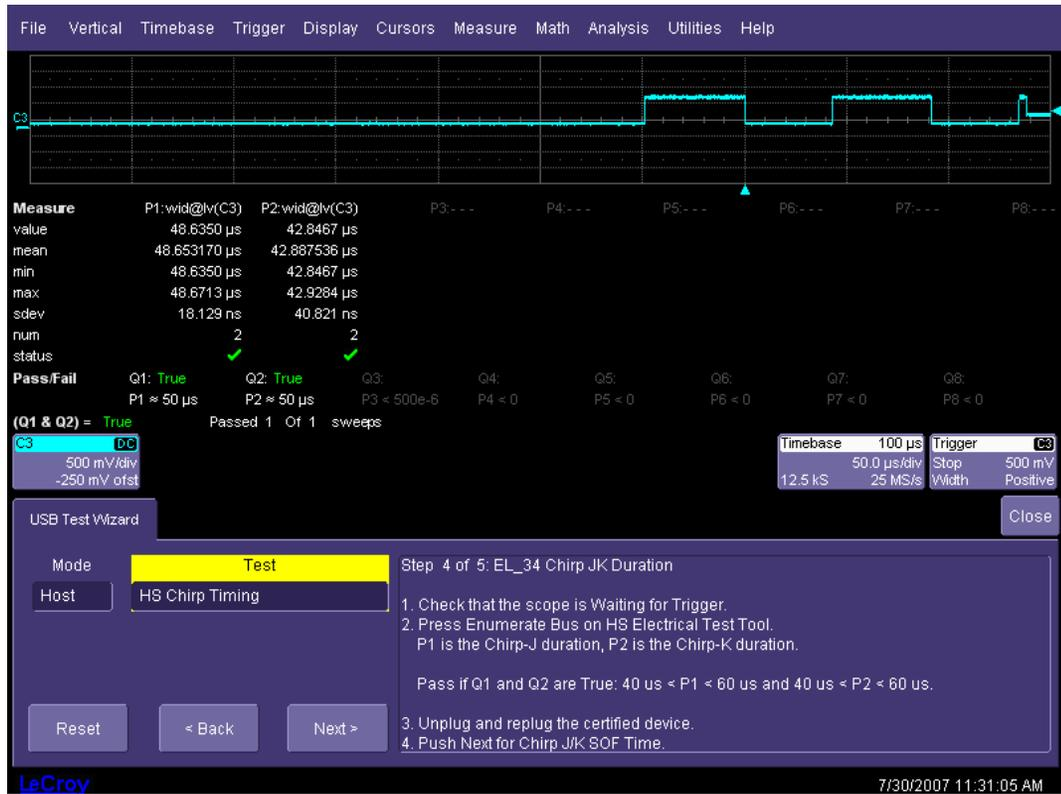
Figure 28. Chirp J and Chirp K Duration
