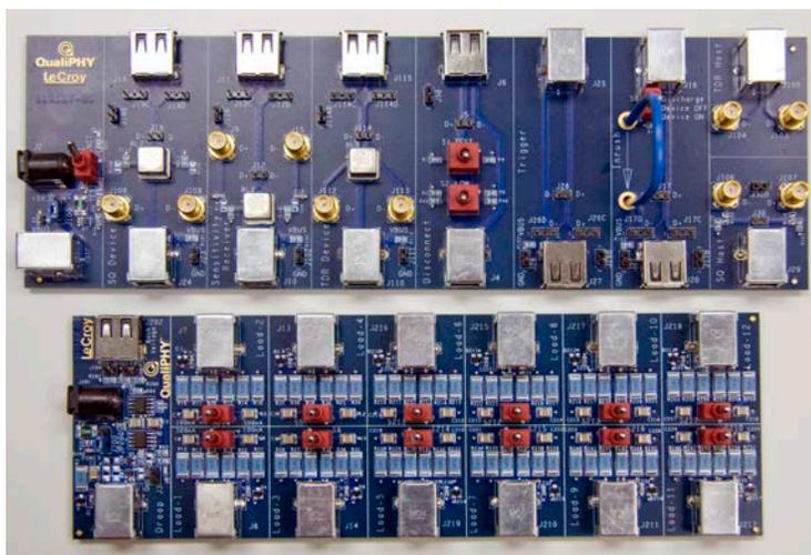
**Figure 1. USB 2.0 Test Fixture (Part Number TF-USB-B)**
