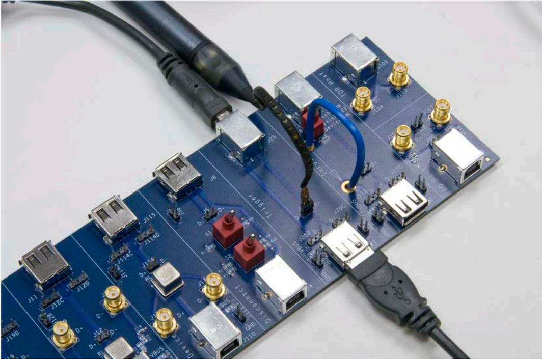
Figure 19. D600ST-SP Connected to the Test Fixture
