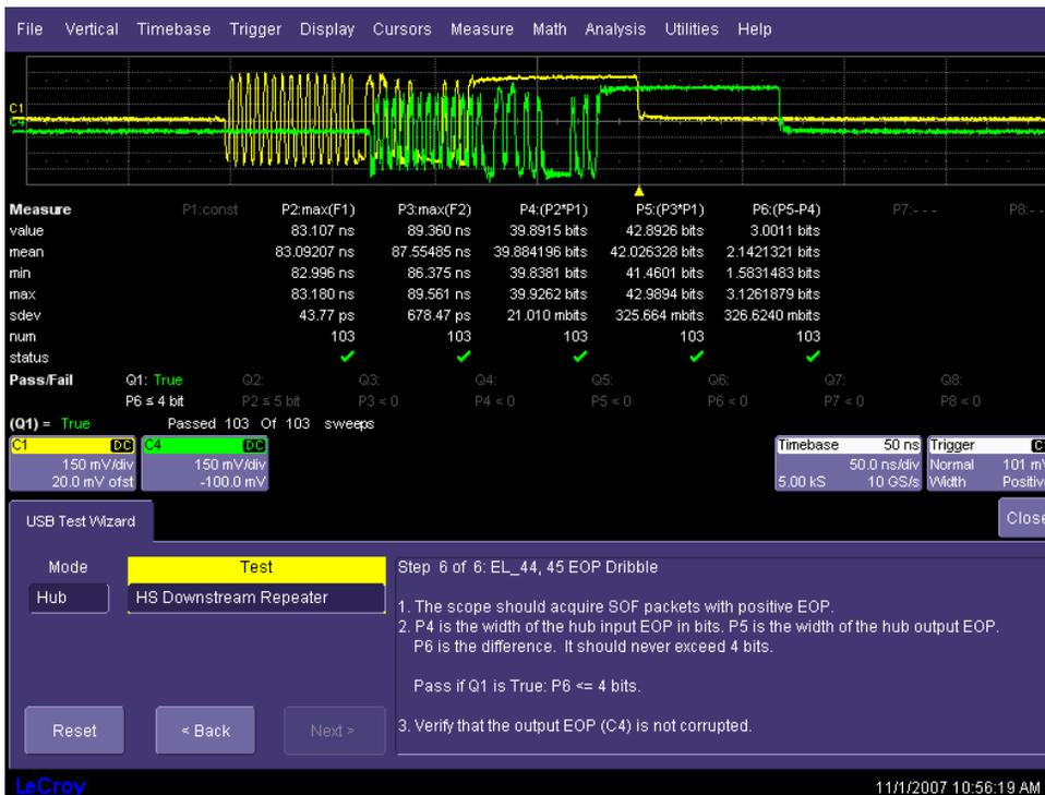
**Figure 44. Hub downstream repeater end of packet dribble**
