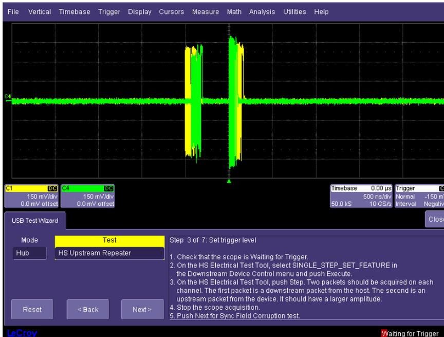
**Figure 37. Initial signal acquisition for hub upstream repeater test**
