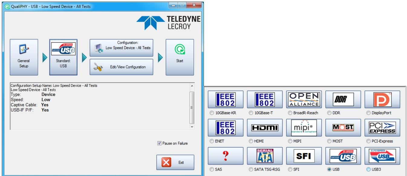
Figure 7. QualiPHY main menu and compliance test Standard selection menu
