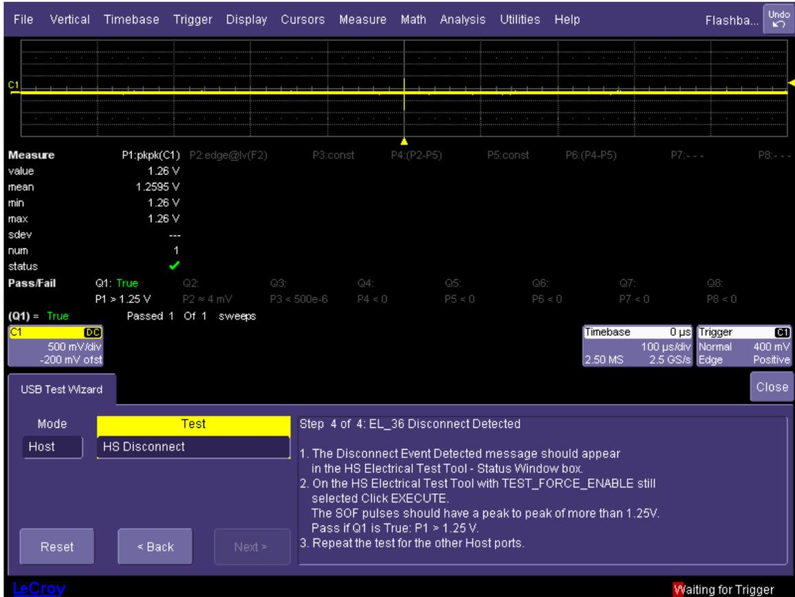
Figure 35. Voltage after disconnect
