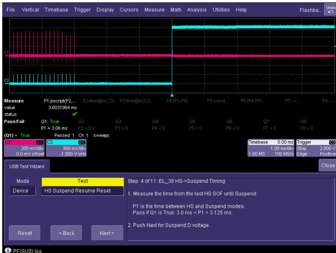
Figure 32. Time from Last Start of Frame to Device Suspend
