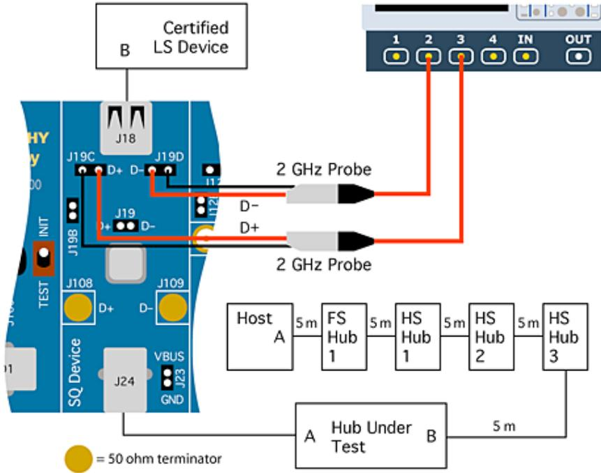
**Figure 60. Hub Low-Speed Downstream Signal Quality Setup**
