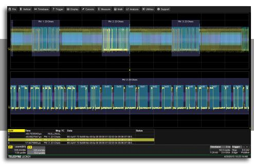
The SpaceWire decode adds a unique set of tools to your Teledyne LeCroy oscilloscope that simplifies the design, debug, and maintenance of SpaceWire systems. The high speed SpaceWire data stream is annotated directly on the physical layer waveforms. Various sections of the protocol are color-coded to make it easy to understand the protocol traffic. The decoder provides an interactive table, search, and zoom to make debugging fast and effective.
