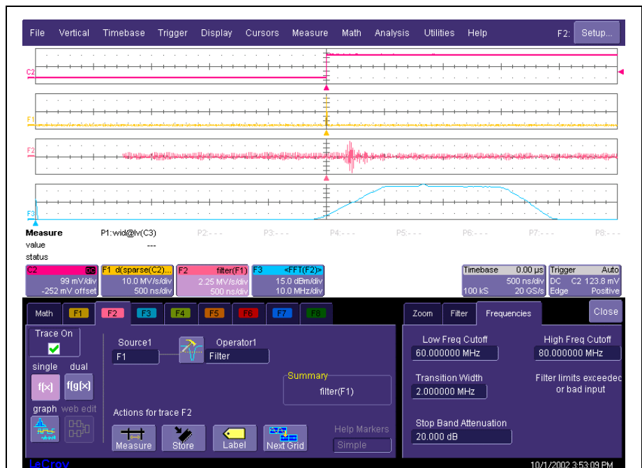
Figure 2 - Filter cutoff frequencies, transition width, and stop band attenuation controls in the DFP2 filter option for the WaveMaster series oscilloscopes
