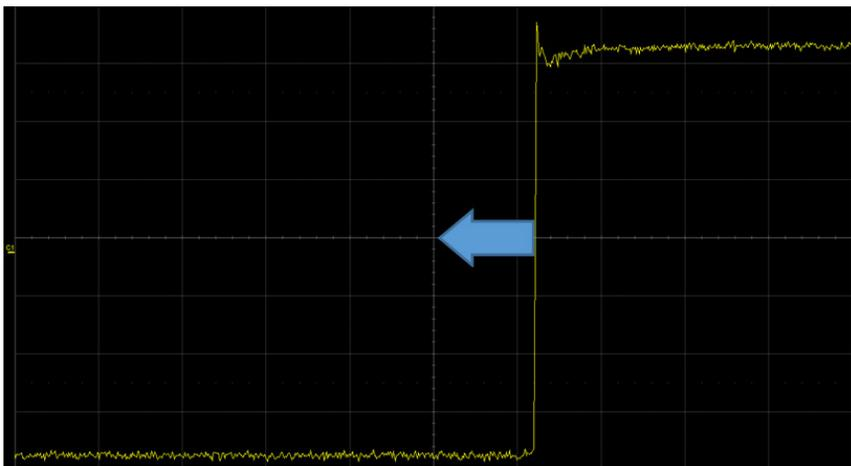
5. Adjust the channel's deskew value so that the 50% rising edge point is centered in time, as shown below.
