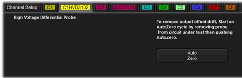
Figure 91: Auto Zero button on Probe dialog.
