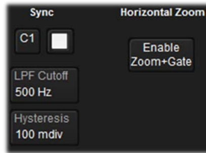
Figure 25: Sync signal setup.
