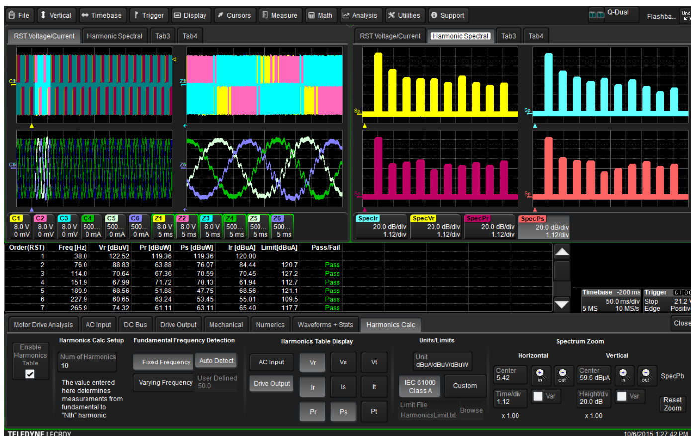
Figure 88: Harmonic Order table and Spectral waveform example.
