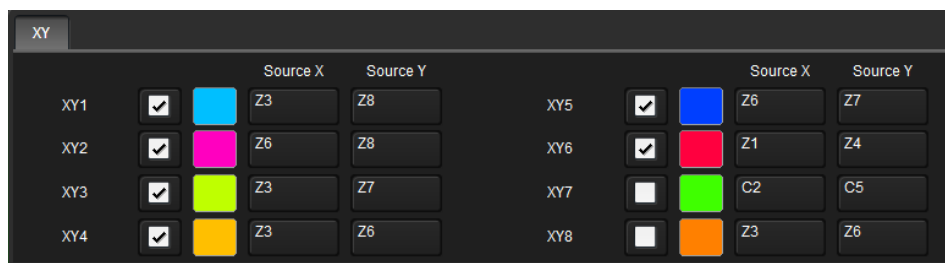
Figure 74: Multiple XY plot definitions using vertical zooms as sources.
