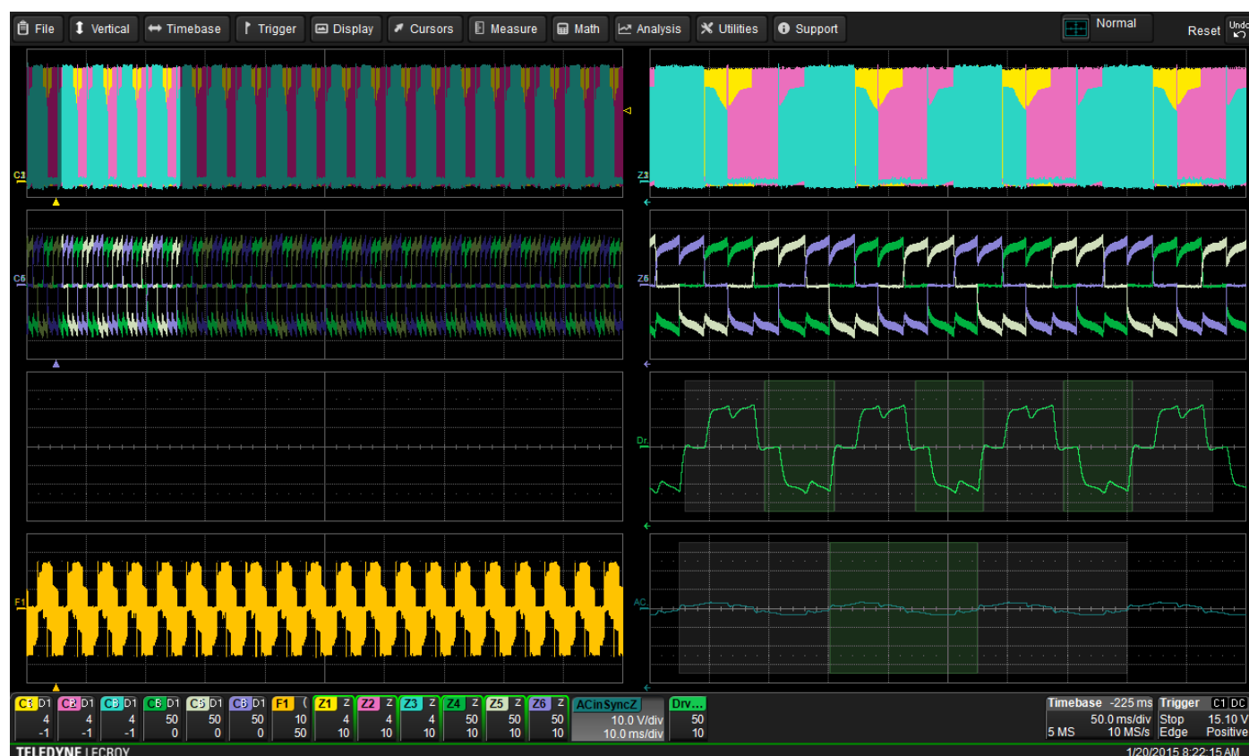
Figure 40: Changing ACinSyncZ source to math function improves periodicity (blue, lower right).
