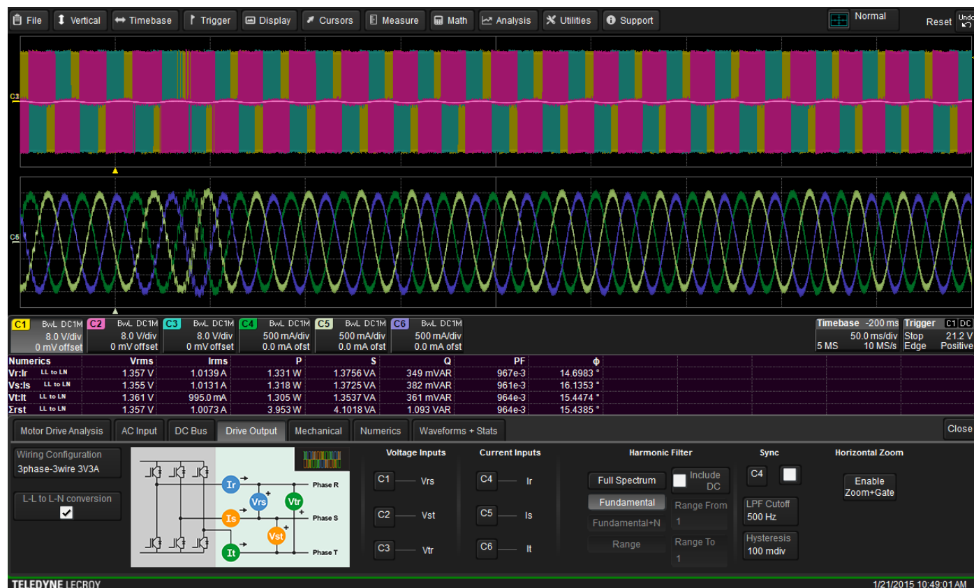
Figure 22: Numerics data calculated for only the Fundamental Harmonic. Note that only the table changes.
