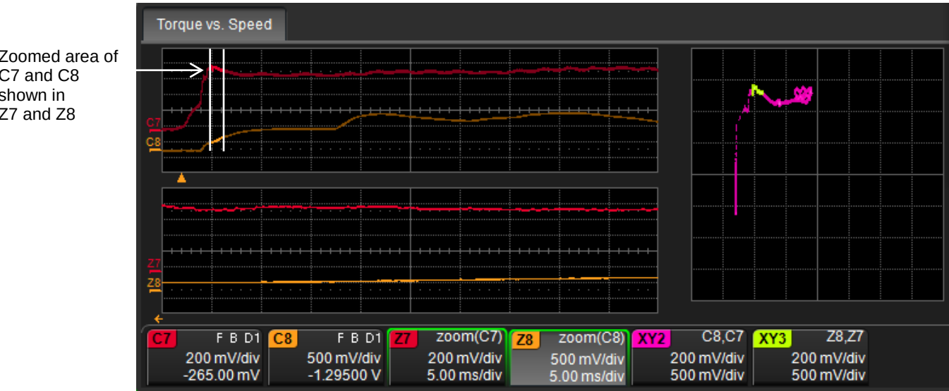
Figure 71: XYDual grid mode selection in tabbed Q-Scope display mode.
