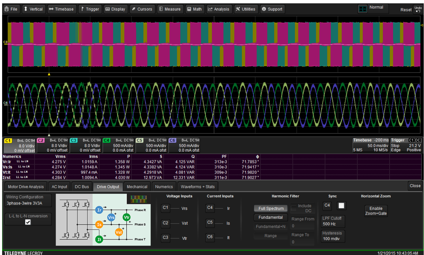
Figure 21: Numerics data calculated for the Full Spectrum.
