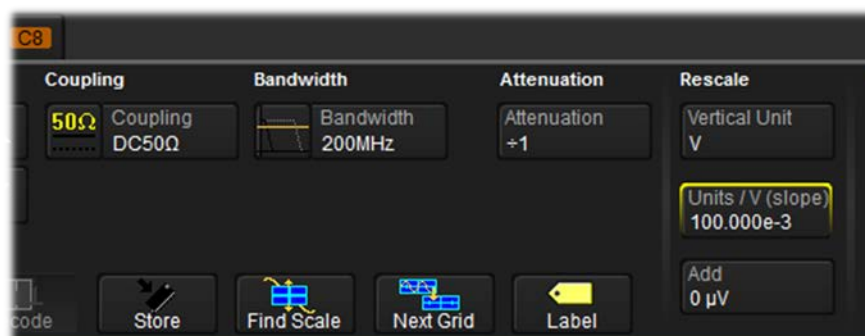
Figure 5: Define input signal characteristics on the Channel (Cx) dialog.
