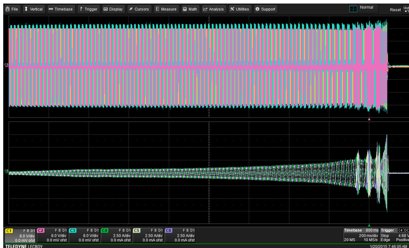
Figure 34: Initial display of input source waveforms for sine-modulated three-phase drive.
