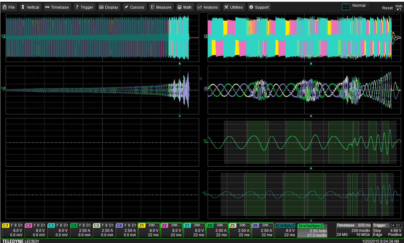
Figure 37: Adjusting filters reveals DriveOutSyncZ is the better choice Sync signal.
