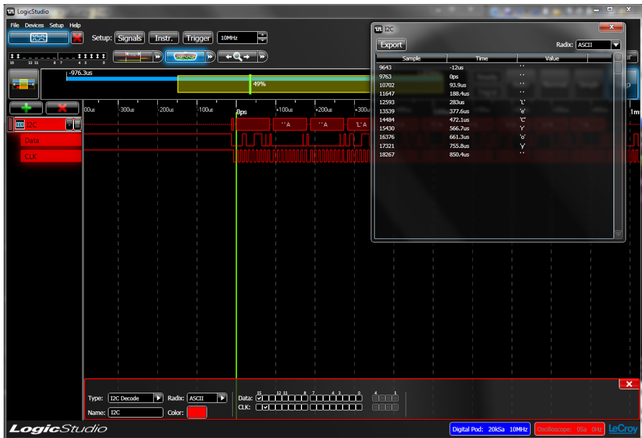
Figure 7: The I2C decode display with the data table pop up
