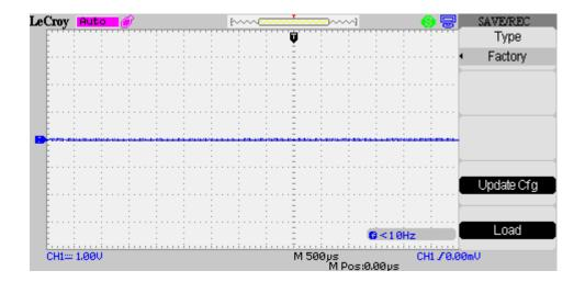
At any time the menu on the right-hand side of the screen can be removed/restored by pressing the front panel MENU ON/OFF button.
