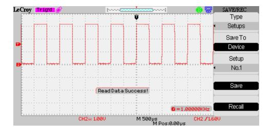
To prevent the trace being overwritten the scope is switched to Stop mode. Recoonect the probe and press RUN/STOP to restart the acquisition.
