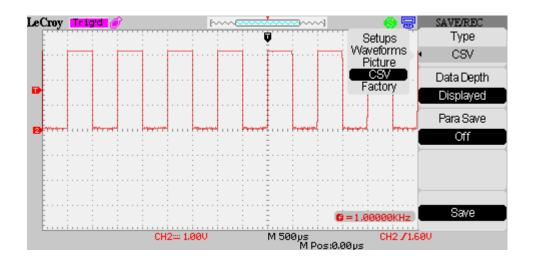
**Step 7:** Repeat Step 4 but this time select Save To as File. Use the filename SU00001. Now try to load the file back in. Note: to use the Load button first select Save, scroll to the correct file and then press Load. Setup files have the extension .SET
