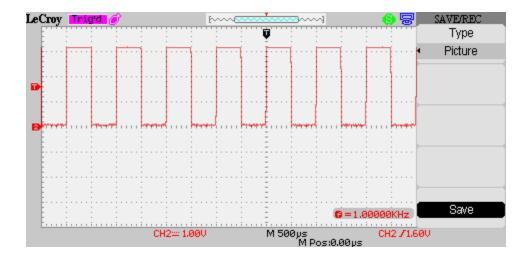
**Step 6:** Press the menu Save button or the front panel PRINT button. After a few seconds the listing of the USB memory is shown on the screen. Picture files can only be saved so the Load button is greyed out.
