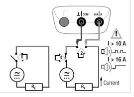
5.7.3 Direct and Pulsating Current Measurement with Current Clamp Sensor, A DC and A (DC+AC)
