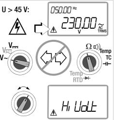
ment is disabled. The measuring function is not switched until dangerous touch voltage is no longer applied to the input. If the instrument switches itself off in the event that hazardous touch voltage is applied (during memory mode operation with large sampling period), the high-voltage warning symbol remains visible at the display.
