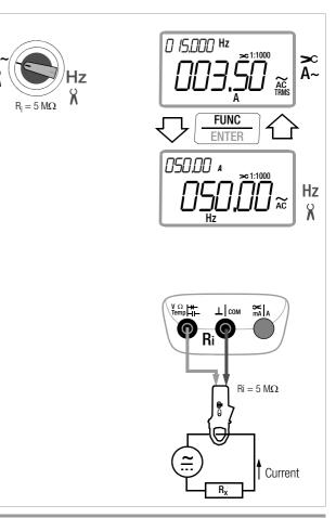
5.7.5 Alternating Current Measurement with Current Clamp Transformer, A AC and Hz  $\,$
